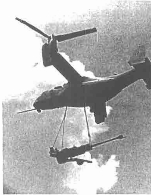
Figure III-9. MV-22 Lifts a Lightweight Towed Howitzer
